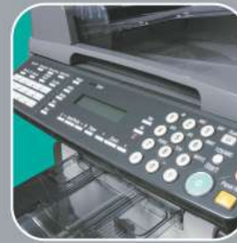
Fax-copy control panel with easy-to-use fax/scan/copy buttons and LCD screen
